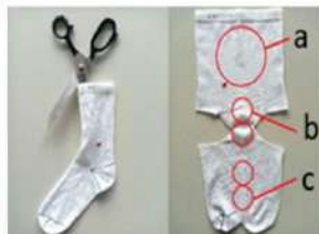
Sampling of socks: a) for testing of propensity to surface pilling; b, c) for testing of abrasion resistance
