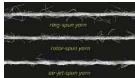
Figure 3. Structure of ring, rotor and air-jet spun yarns
