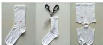
Figure 5. Preparation of sock for water vapor absorption and air permeability test
