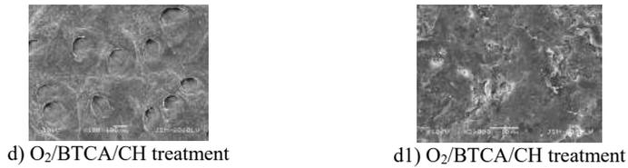
**Fig. 2.** SEM images of chrome tanned leather with 100x (left) and 2000x (right) magnifications: a, a1) untreated; b, b1) O<sub>2</sub> plasma pretreated; c, c1) O<sub>2</sub>/BTCA treatment and d, d1) O<sub>2</sub>/BTCA/CH treatment
