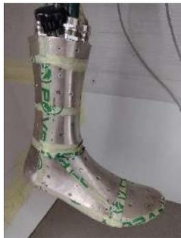
Figure 1: Bare thermal foot model hanging inside a climatic chamber
