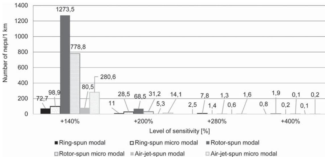
Figure 11: Number of neps of modal and micro modal ring-, rotor- and air-jet-spun yarns for different levels of sensitivity
