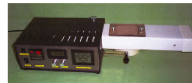
Figure 1: PERMETEST - device for non-destructive determination of water vapour and thermal resistance, by Sensora Instruments [17]
