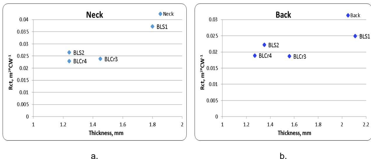
**Figure 2** Graphical view dependence of thermal resistance on the thickness: a) samples from neck parts, b) samples from back parts
