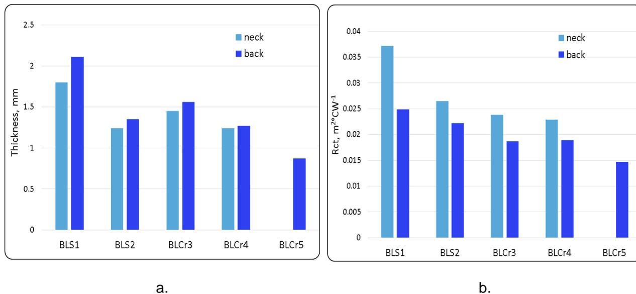
**Figure 1** Graphical view of results measured on the samples from neck and from back parts of the leather: a) thickness, b) thermal resistance
