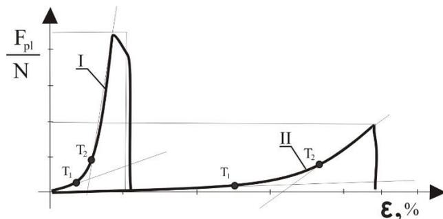
Figure 2. Force-elongation diagram of double knit jersey fabric; I) in wale direction and II) in course direction;  $T_1$  – end of the elastic area,  $T_2$  – point of inflection, beginning of the elastic area
