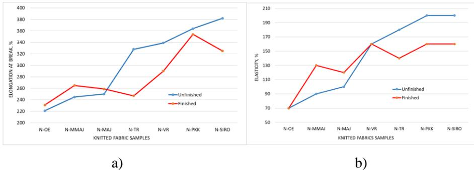
Figure 4. Elongation properties of unfinished and finished knitted fabrics in course direction – transverse; a) up to breakage, b) elastic area
