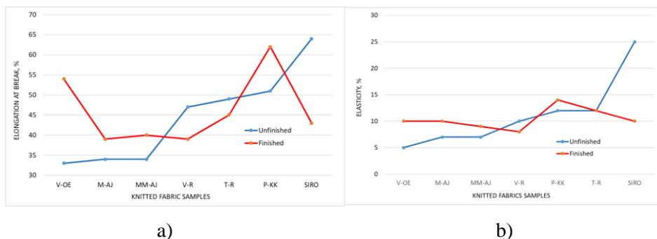
Figure 5. Elongation at break of the finished and unfinished fabrics in wale direction – longitudinal; a) up to breakage, b) elastic area
