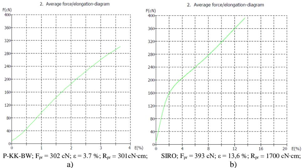
Figure 3. Elongation properties of yarns: a) ring cotton yarns, b) viscose Siro yarns
