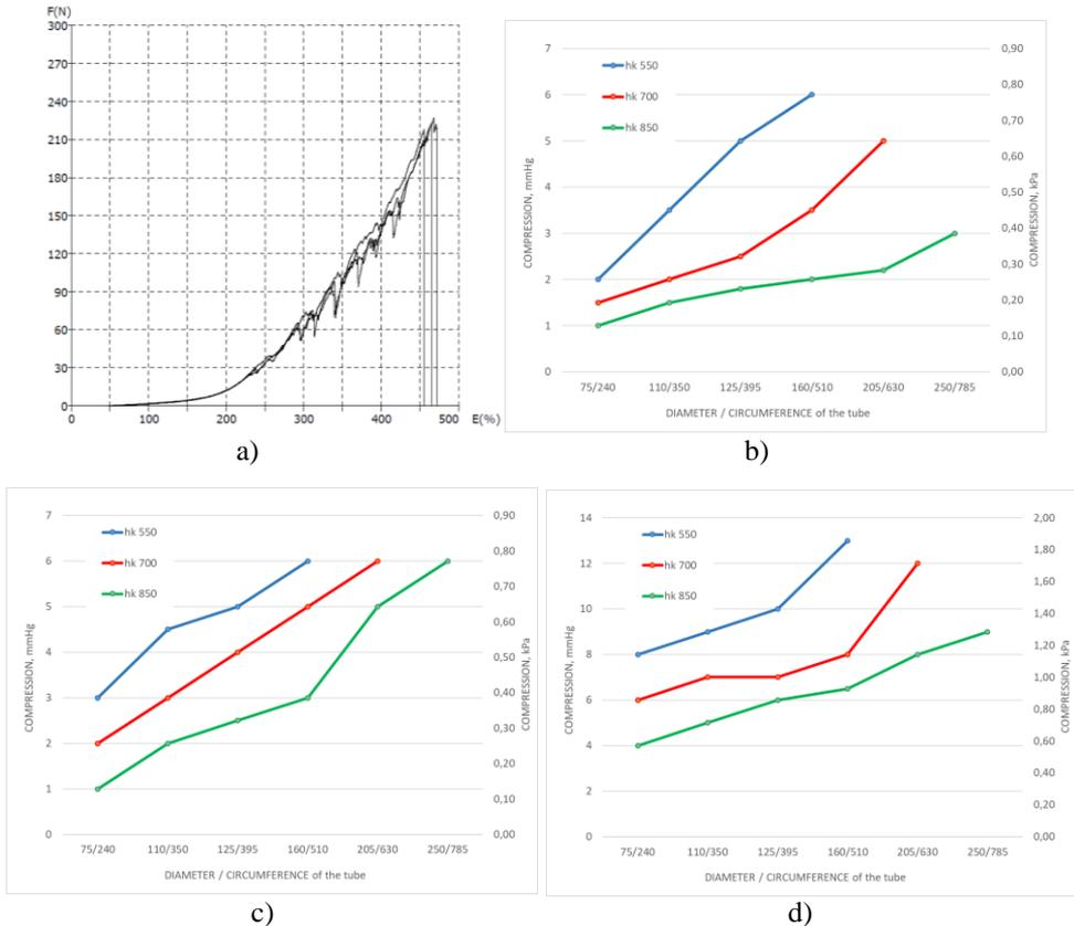
Figure 3. The Results of stretchability and compressibility measuring of the tubular knitwear samples;
