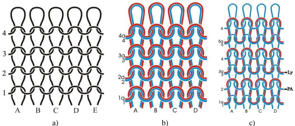
Figure 1. Basic knit structures used to make fine women's hosiery: a) plain structure, b) basic plated structure, c) partial plating – plated in every other row
